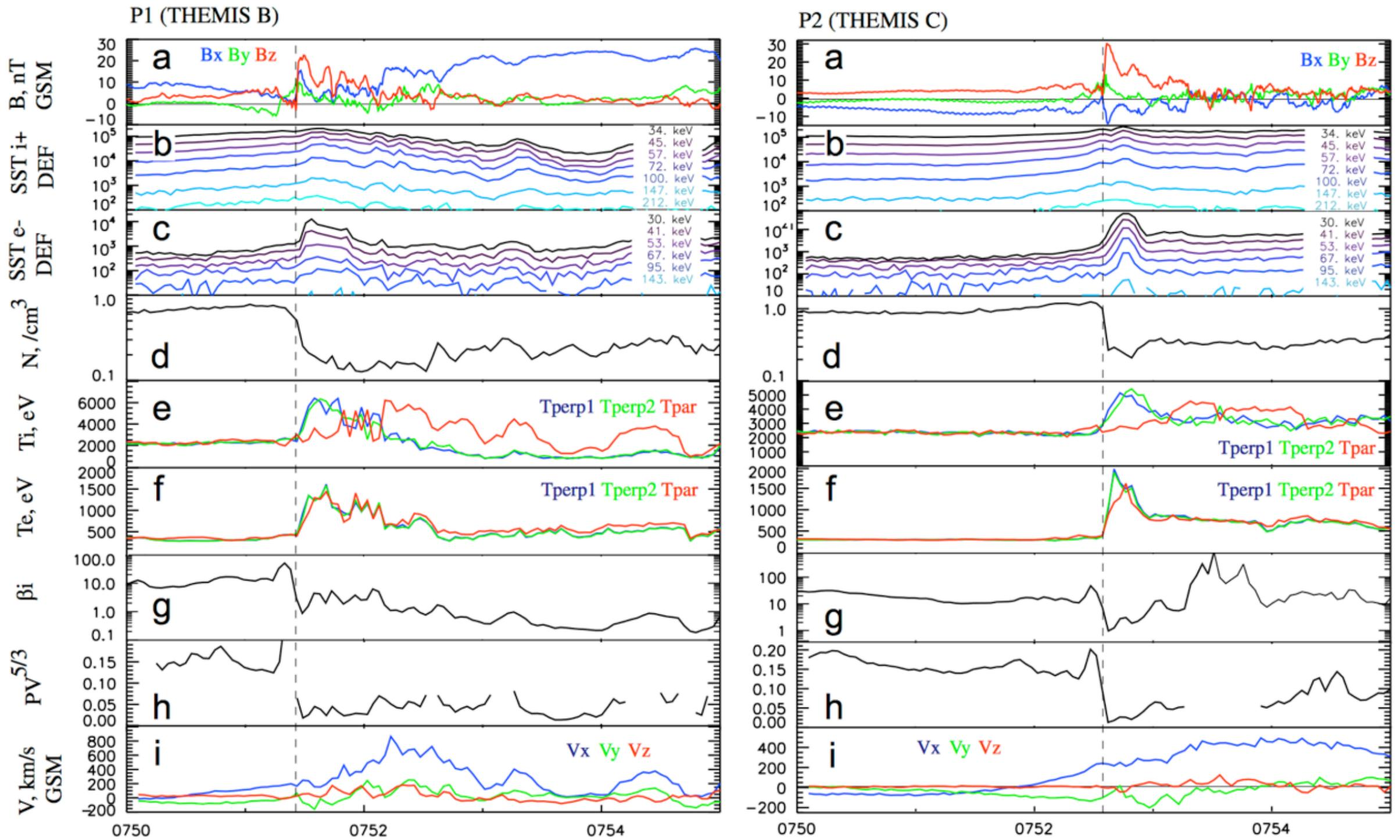
This is a typical bursty bulk flow, with an extended flow  $> 100$  km/s depleted density, increased temperature (and decreased entropy)
